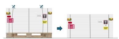
**CAUTION:** If you must tilt the unit on its side, keep it in its outer box, place the side labeled "**Heavier Side**" on the bottom, and use a dolly or hand truck to move it. Remove the outer box only once the unit is in its final installation spot.
