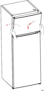
18. Attach the freezer door by inserting it onto the pin, pushing down and toward the unit.
