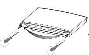
15. Switch the bottom freezer door hinge to the opposite side.
