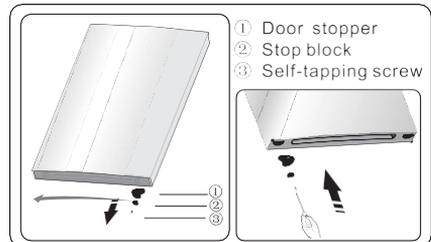
8. Loosen the screws used to affix the middle hinge and remove the middle hinge. Then remove the lower door.
