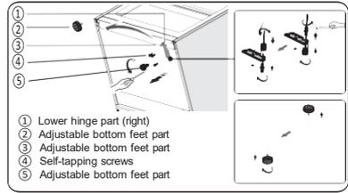
12. Remove part (3) from the lower hinge pin, loose out the lower hinge pin, change it to the reverse hole site, and then tighten into position, then install part (3) on the lower hinge pin.
