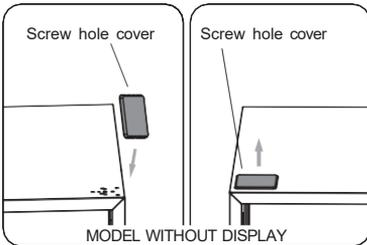
6. If the refrigerator with a display on the door, remove part ① from the top left side of the upper cover and take out part ②. Then remove part ③ and put part ④ into the top right side of the upper cover. Refer to the above operation, install part ③ and part ④ on the top left side of upper cover. Install part ① of the top right side of the upper cover. When the refrigerator is without a display on the door, skip this step.
