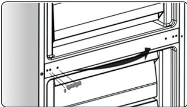
11. Tip the refrigerator backward and remove part (2).
