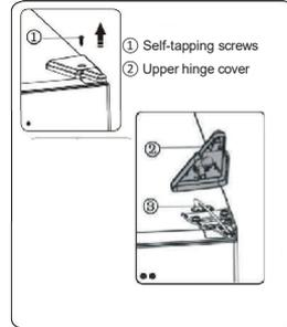
3. Remove screws ① and hinge ②. When the refrigerator with a display on the door, you need to pass connector ③ through the hole of the hinge ②. (Hold the upper door by hand when installing).
