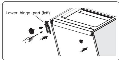
14. Slot the lower door onto the bottom hinge pin and hold it in position. Turn the middle hinge 180°, change the washer on the axis to the lower side, adjust the middle hinge to the appropriate position, and then install it ensuring the lower door is in place.
