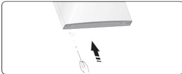
10. Change screw hole covers on the middle cover plate from left to right (as shown in the figure below).
