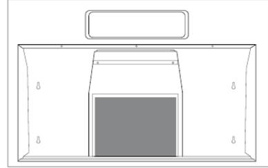
2. **For ducted installation:** Install the grease filters.
