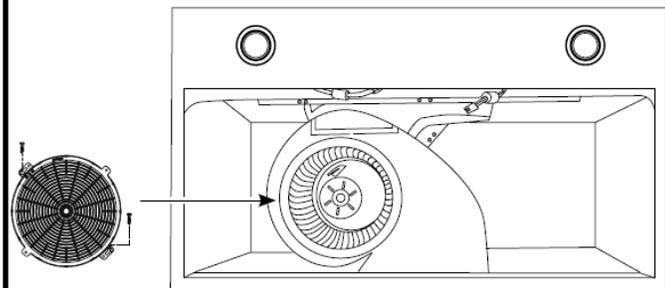
2. **For vented installation:** Install the grease filters.
