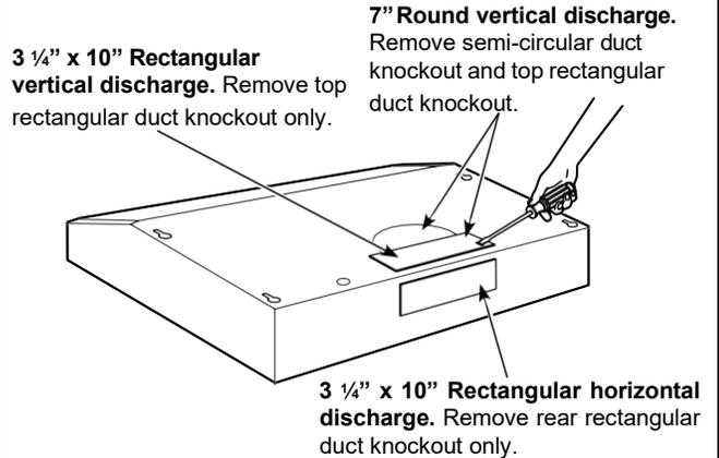
**NOTE:** If the hood is to be installed in a recirculation, non-vented ductless manner, do not remove any venting knockouts.
