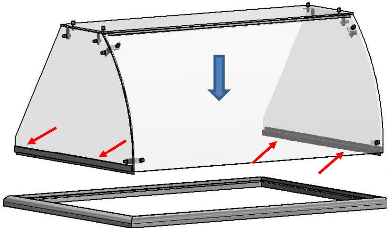
Place the sneeze guard on the freezer, press the sides to the inner side of the box, and fasten the sides to the freezer
