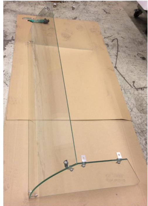
Fasten the right hand Side glass to the Front glass with 2 x screws no.6, 4 x plastic washers, 2 x nuts
