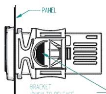
Instrument XR30CH shall be mounted on vertical panel, in a 29x71 mm hole, and fixed using the special bracket supplied. The temperature range allowed for correct operation is 0÷60 °C. Avoid places subject to strong vibrations, corrosive gases, excessive dirt or humidity. The same recommendations apply to probes. Let air circulate by the cooling holes.
