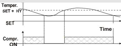
In case of fault in the thermostat probe the start and stop of the compressor are timed through parameters "**CO<sub>n</sub>**" and "**CO<sub>F</sub>**". Defrost is performed through a simple stop of the compressor. Parameter "**IdF**" controls the interval between defrost cycles, while its length is controlled by parameter "**MdF**".
