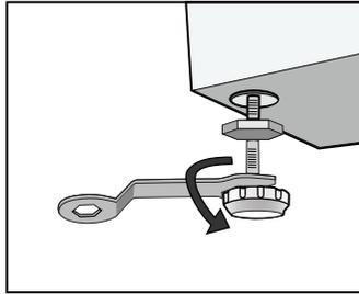
3. Ensure the positioning status of washing machine. Loosen the lock nut with spanner and turn the leg with hand until it closely contacts with the floor. Press the leg with one hand and fasten the nut closely to the cabinet with the other hand.
