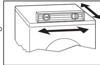
4. After being locked properly, press four corners again to make sure that they have been adjusted properly. If it is still unstable, it has to repeat Steps 2 and 3.
