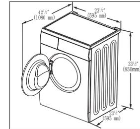
The dimensions shown are for the recommended spacing. Custom dercounter installation
