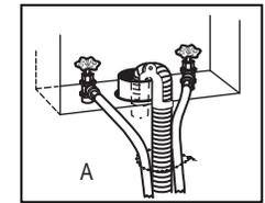
Capacity can be no less than 17 gal. (64 L) per minute. The top of the standpipe must be at least 60cm high and no higher than 100cm from the bottom of the washer.
