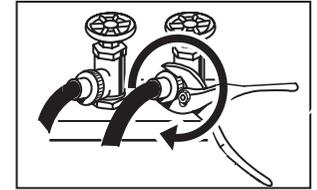
Note: after connection, if there is any leakage with hose, then repeat the steps to connect inlet pipe. The most common type of tap shall be used to supply water. If tap is square or too big, then standard tap shall be changed.
