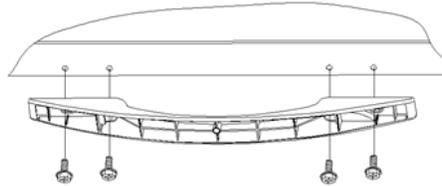
**NOTE:** There is a notch cut into the handle, designed to accommodate the freezer lock. The handle must be positioned with the notch on the right-hand side, facing down.
