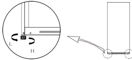
Turn the feet clockwise to raise the refrigerator and turn the feet counterclockwise to lower the refrigerator.
