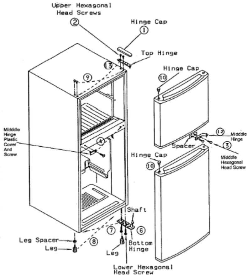
1. Remove the hinge cap by twisting it off.
