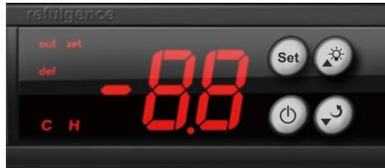
The control panel is located on the back, interior wall, in the upper right-hand corner. Under normal operation, the LED display shows the internal temperature of the cabinet. If you have any other questions regarding the operation of this unit, please call our Customer Service Department at **1-800-932-4267** (9:00AM to 5:00PM ET).
