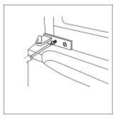
13. Place the upper door back onto the middle hinge. Make sure the door is properly aligned so the seal closes properly, making sure the middle hinge pin fits into the upper hinge hole of the lower door. Tighten the bolts.
