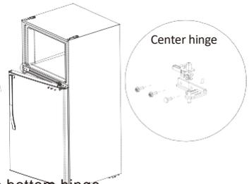
5. Unscrew screws of the bottom hinge, then remove the bottom hinge from the bottom right side of the refrigerator.
