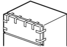
2. Remove the left cover plate and the right top hinge cover, then unscrew SCREWS and remove the right top hinge. Keep the screws to reuse.
