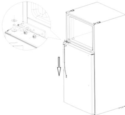
10. Put down the freezer door on the middle hinge vertically, then take out the top hinge and cover of other side from accessory bag, assemble top hinge, hinge cover and hole cover.
