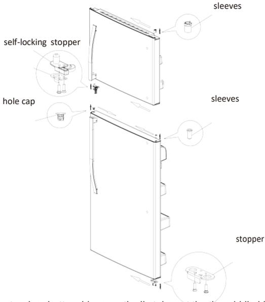
9. Put down the refrigerator door bottom hinge vertically, take out the middle hinge of the other side from the accessory bag then assemble the middle hinge on.
