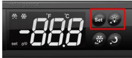
To adjust the temperature, press and hold the SET key for 3 seconds. When the display shows **St**, you can raise the temperature by pressing the LIGHT key or lower it by pressing the MENU ADJUST key, shown below. Press the ❄️ key, or press no key for 30 seconds, to exit. The temperature set-point will be saved automatically.
