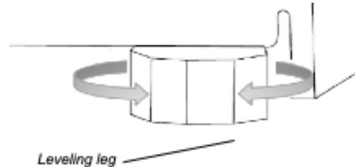
**NOTE:** It is easier to adjust the leveling legs if someone else pushes against the top of the appliance to take the weight off the legs.
