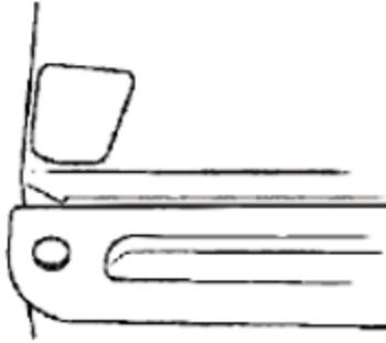
3. Remove the plastic insert on the opposite side of the refrigerator door.
