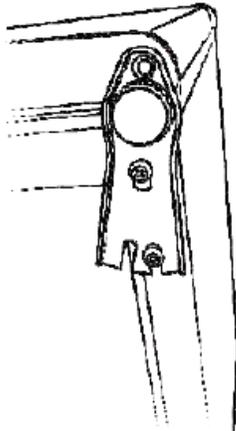
6. Unscrew the two screws holding the bottom door hinge, and carefully move it across to the opposite side.
