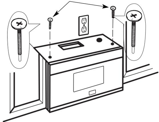
**7** Tighten the outer two screws to the top of the microwave oven. (While tightening screws, hold the microwave oven in place against the wall and the top cabinet.)
