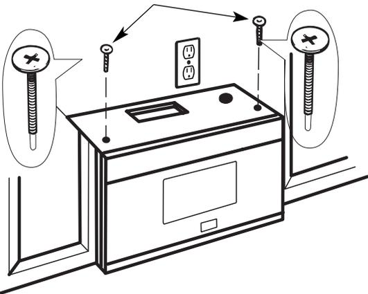
**6** Tighten the outer two screws to the top of the microwave oven. (While tightening screws, hold the microwave oven in place against the wall and the top cabinet.)
