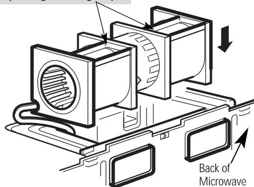
**CAUTION:** Do not pull or stretch the blower unit wiring. Make sure the wires are not pinched, and that they are properly secured.
