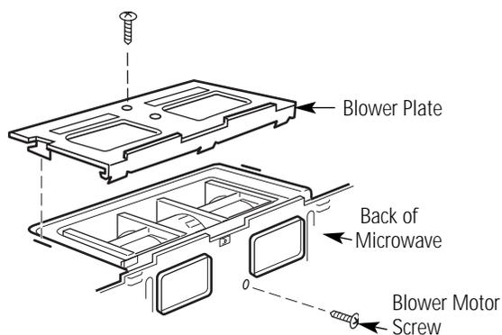
Remove the screw that holds the blower plate to the microwave. Remove and save the screw holding the blower motor to the microwave.
