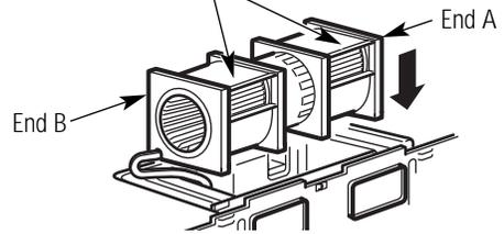
**CAUTION: Do not pull or stretch the blower unit wiring. Make sure the wires are not pinched, and that they are properly secured.**
