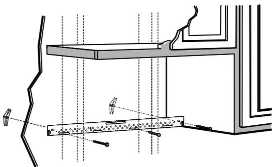
Attach the plate to the wall using toggle bolts. At least one wood screw must be used to attach the plate to a wall stud.
