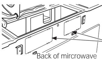
**Knockout Plates:** Snip all 4 webs on each knockout panel and remove the metal knockouts for rear airflow. Please take care to remove any sharp edges created from removing the knockout plates.
