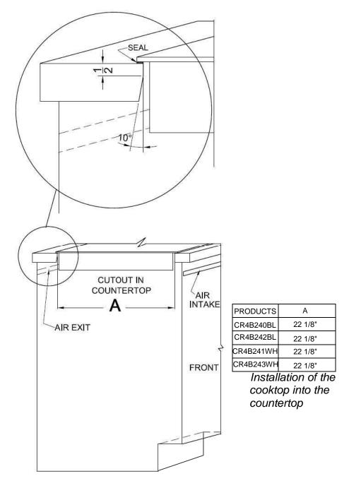
Place the cooktop in the cutout opening and press firmly on all sides to seal the frame into the bedding compound. The sealant will hold the cooktop firmly in place on the countertop.
