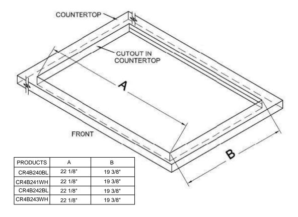
Note: When making the countertop, put a radius at the corners of the cutout (a radius of ½" is typical). This will keep the countertop from cracking. Follow the countertop manufacturer's instructions regarding the minimum corner radius and reinforcement of corners.
