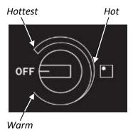
There is a light associated with each of the control knobs that provides an indication of burner operation and a hot surface. When a control is in the ON position, the red light is lit indicating which burner is on and is therefore too hot to touch. Do not place articles other than cookware on the cooking surface while this light is glowing.
