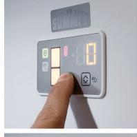
Again, press and hold both the temperature adjustment button and the blank button for 3 seconds
