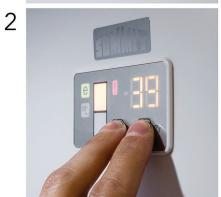
Press both the temperature adjustment button and the blank button and hold them for 3 seconds
