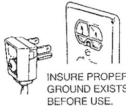
Do not use an extension cord to connect this appliance. If the power supply cord is too short, have a qualified electrician or serviceman install an outlet near the appliance.
