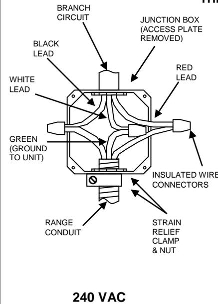
1. Remove the access plate to gain access to the electrical junction box.
