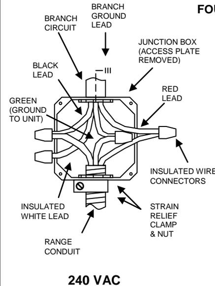
1. Remove the access plate to gain access to the electrical junction box.
