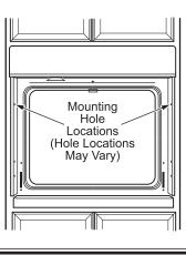
The screws must be a minimum of 6 mm (1/ 4") from the front of the cutout.
