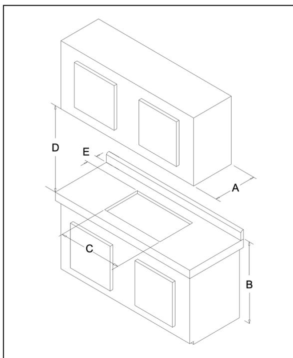
**NOTE:** Do not install closer than 1/2 in. (12 mm) from any adjacent surface.
