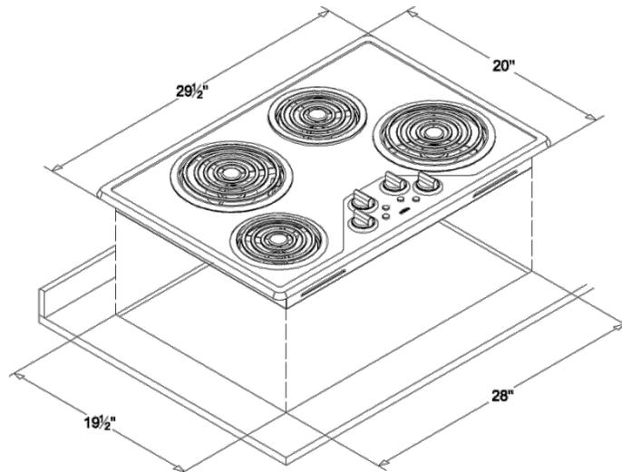
**NOTE:** When making the countertop, radius the corners of the cutout (1/4" radius is typical). This will prevent cracking of the countertop. Follow the countertop manufacturer's instructions regarding the minimum corner radius and reinforcement of corners.
