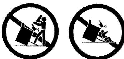
To reduce the risk of tipping, the range must be secured by properly installed anti-tip bracket provided with the range. Please refer to the anti-tip bracket installation instructions for proper installation.
