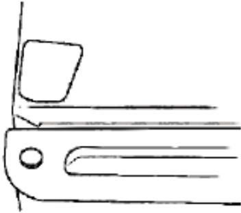
4. Remove the adjustable foot at the bottom of the fridge and set aside.
