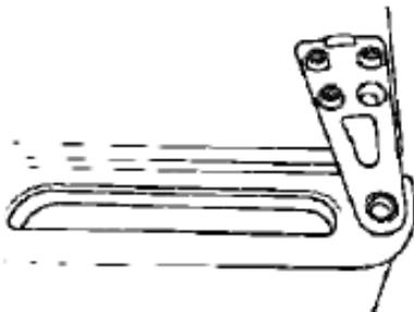
3. Remove the plastic insert on the opposite side of the fridge and door. Now fix the top door bracket to this side using the screws that were previously removed. Replace the plastic hinge cover.
