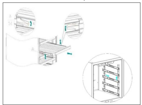
First remove all wine bottles from the shelf and pull it out as far as you can. Simultaneously press down the left lever on the sliding shelf and press the right one up, pulling the shelf out at the same time. Next, push up on the shelf to release the front hook from the shelf bracket. Then just pull the shelf out.
