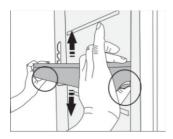
The height of the door bins can be adjusted without having to remove the bins from the appliance. Simply pull the two levers on each side of the bin towards you and slide the bin up or down.
