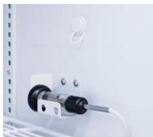
Temperature sensor in glycol bottle
