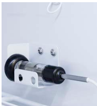
Temperature sensor in glycol bottle
