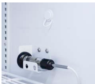
Temperature sensor in glycol bottle
