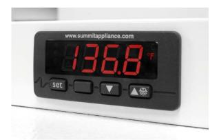
When the cabinet reaches 140°F, the heating element will turn off (the red light goes out), then turns on again when the cabinet temperature drops to 135°F. This condition will continue until the equipment is turned off intentionally or:
