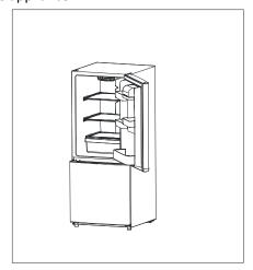
3) Remove the screws from the middle hinge. Lift the refrigerator door up and away from the appliance.
