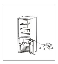
4) First loosen the screws and remove the right hinge and gasket. Take out the left hinge and remove the screws fixed to the left hinge and shim. Finally attach the left hinge and gasket using the screw holes on the left side of the refrigerator.
