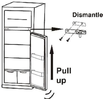
Remove the screws from the middle hinge. Lift the refrigerator door up and away from the appliance.
