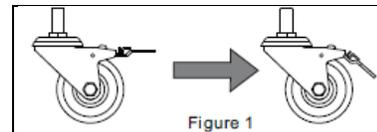
Install the two universal wheel washers at the front of the cabinet base, and then install two universal wheels without foot brakes. Next, install the two universal wheels with foot brakes at the back of the cabinet base. Once installed these rear wheels will keep the unit from moving if you step on the foot brakes (See Figure 2):
