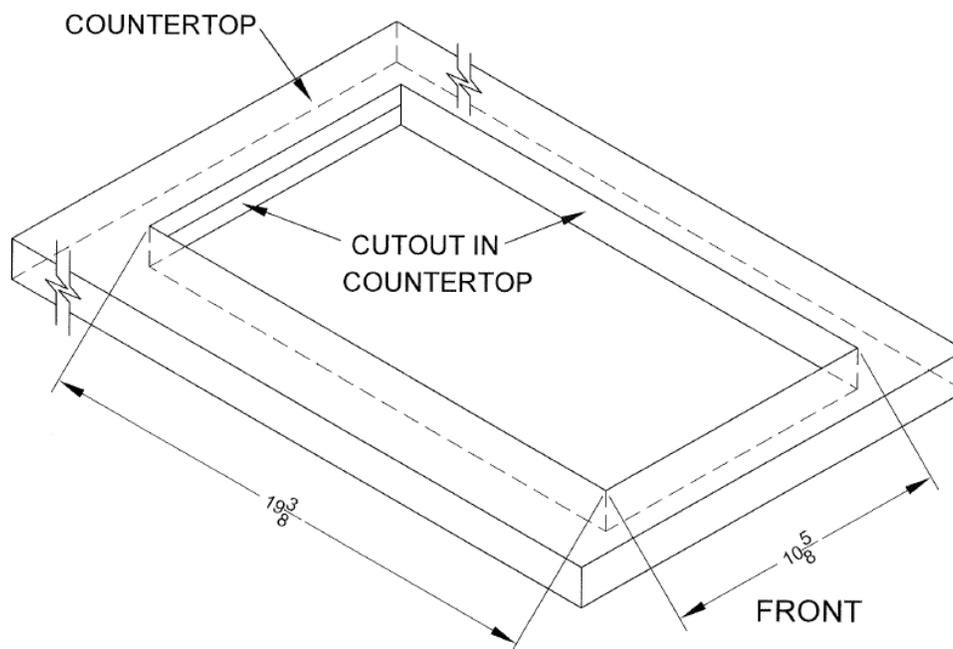
**Note:** When making the countertop, put a radius at the corners of the cutout ( $\frac{1}{4}$ " radius is typical). This will keep the countertop from cracking. Follow the countertop manufacturer's instructions regarding the minimum corner radius and reinforcement of corners.
