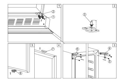
5. Screw the alternative left top hinge (6), included in the fittings, on the left-hand side of cabinet. (Fig. 3)
