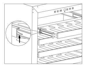
with the tracks in the cabinet. Ensuring an even track engagement on both sides, gently push the shelf into the cabinet until it stops.
