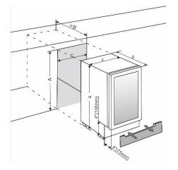
**NOTE:** When pushing the appliance into the niche, make sure that the mains cable does not get trapped.
