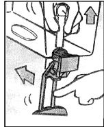
6. Pull out the tap lock pin to unblock the dispensing lever.
