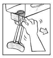
7. The tap body can then be removed from the container.
