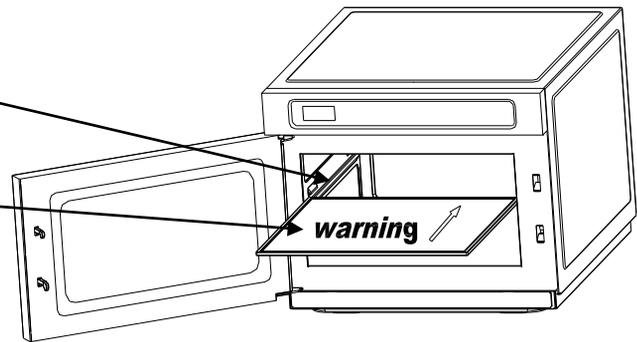
3. Be sure the ceramic board has been pushed all the way to the back of the cavity. If you do not install it correctly, the door cannot be closed.
