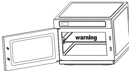
2. Gently pull the ceramic board out of the cavity along the grooves. To prevent damage, do not force or shake the board as you pull it.
