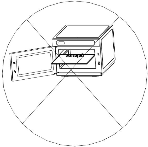
To remove the ceramic board from the cavity:
