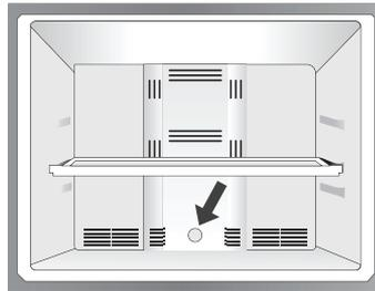
By turning the control to the left, the air flow to the cooler will increase, delaying the freezing process according to the following guide:
