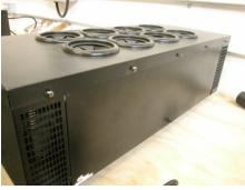
Secure the back of the cover with 5 screws. Installation is complete.
