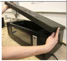
Remove 12 screws around the cover using a Phillips screwdriver.
