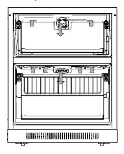
Blocking the vents will restrict the air movement and cause temperature and moisture problems.
