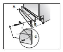
If the enclosure height is above 33-1/16" (840mm), use "o" and "p" labeled toe kicks together. Make sure the slotted toe kick "p" is on the outside so you can adjust height of the toe kick. Installation should be done following the steps illustrated in the figures **A**, **B** and **C** respectively.
