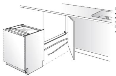
**CAUTION** Make sure all hoses and electrical wire are pulled through the side opening of the cabinet, no hoses are kinked and all slack is taken out as shown in this figure.
