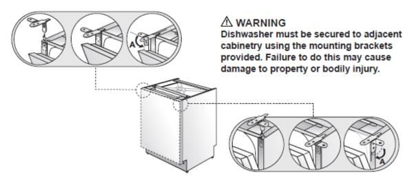
Place the two mounting brackets into the top corners of the dishwasher.
