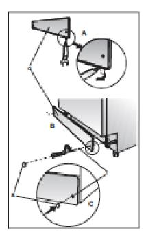
Lock the toe kick brackets as shown with the plastic tab in Figure **C** by pushing the plastic tab on the dishwasher into the teeth of the bracket (**C**).
