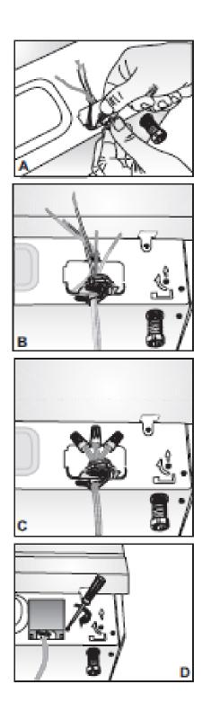
Install a strain relief (not supplied) into the opening on the kick plate. (Figure A)
