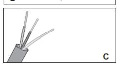
Remove 2-15/16" – 3-15/16" (75mm – 100mm) of the cable's outer casing, and then remove  $\frac{3}{8}$ " –  $\frac{1}{2}$ " (9mm – 13mm) of insulation from each wire (Figure **C**).
