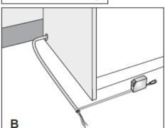
To the right side, position the cable extending approximately  $5\frac{1}{2}$ " (140mm) (Figure **B**).
