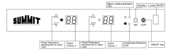
**ON/OFF Key** turns the wine cellar on and off. It should be in the OFF position when the unit is being plugged in to a power source or disconnected from that source.
