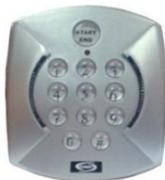
password is lost, press the
