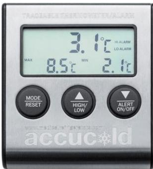
Every MED unit is equipped with a Thermometer/Alarm that simultaneously displays minimum, maximum and current interior temperatures and provides a visual and audible signal when the temperature inside the unit falls outside the set temperature range.
