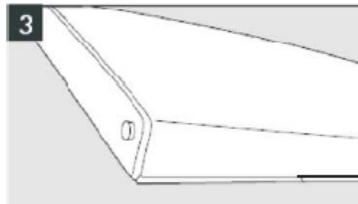
4. Remove the hinge bushing at the top of the door and swap it with the blank on the other side. Repeat with the bushing and blank on the bottom of the door.
