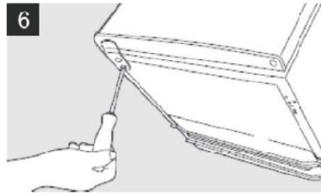
7. Check that door is aligned horizontally and vertically and that the seals are closed on all sides before finally tightening the bottom hinge. Re-adjust the leveling.
