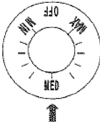
*Normally the Temperature Control Knob should be set at the **MED** position.*
