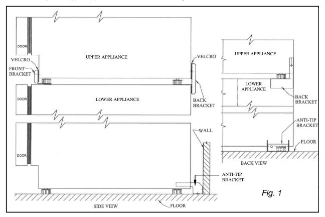
Before stacking the two appliances, the Anti-Tip Bracket should be screwed into place. Follow these instructions:
